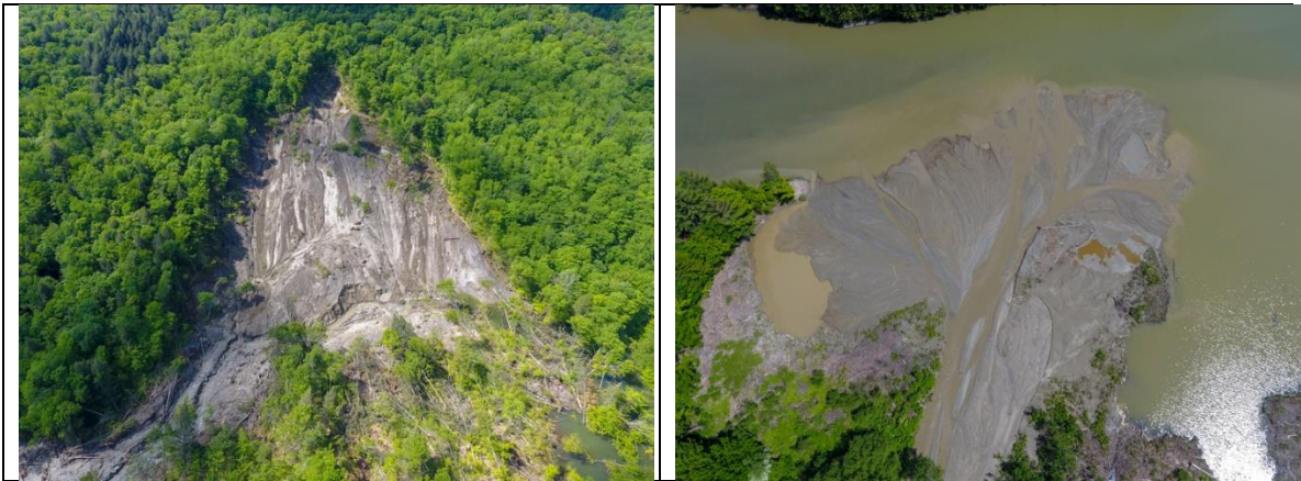
Figure 1. Drone image of the 12-acre landslide at Cotton Brook, Waterbury, VT (image from VTRANS). Figure 2. 2.5 acre delta formed in the Waterbury Reservoir due to sediment from the landslide.
